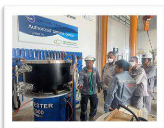
Annual inspection & calibrate Pressure Vacuum Relief Valve at site Project
