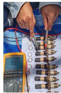
Check and loop test conductivity probe For HP/LP drum (HRSG52) Project
